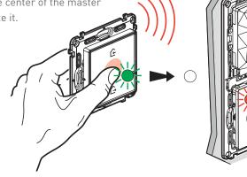
$\rightarrow$  Its LED flashes green then turns off.  $\rightarrow$  The LED of your connected gateway also turns off.
