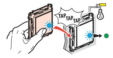
The LEDs of the 2 products flash blue and then light up in solid blue. The wireless control indicator goes off and the connected switch indicator turns green.
